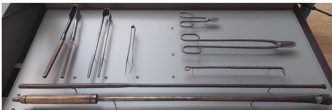
Figure 52. A collection of glassblowing tools at the museum of CNAM.
